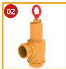
Overpressure Safety Valve - 1 1/4 Code 5100200009 Setting range: +0,3 bar / +1,5 bar Working temperature: -20°C / +90°C Thread: G 1 1/4 Weight: 0,94 kg
