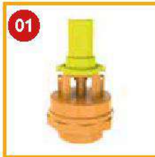
01 Vacuum Relief Valve 1"1/2 Code 5100200012 Setting range: -0,3 bar / -0,8 bar Working temperature: -20°C / +90°C Thread: G 1"1/2 Weight: 0,65 kg
